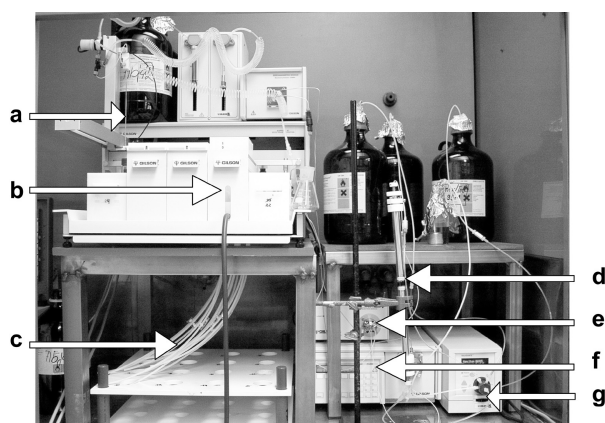
Figure 2. ASPEC XLi system with some adjustments and structural alterations to clean-up samples for the PCB and PCDD/PCDF analysis: SPE unit (left), and additional equipment for the chromatography with activated charcoal (right); a: injection needle with a low pressure valve and a ventilated needle; b: special and new built racks to collect the different fractions; c: special Teflon funnels connected to Teflon tubing; d: LC glass column filled with activated charcoal; e: switch valve to change the flow direction; f: HPLC pump; g: six-point valve connected to the HPLC pump for the different solvents.
